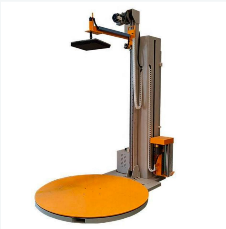
Electric version | Top-press wrapping station
