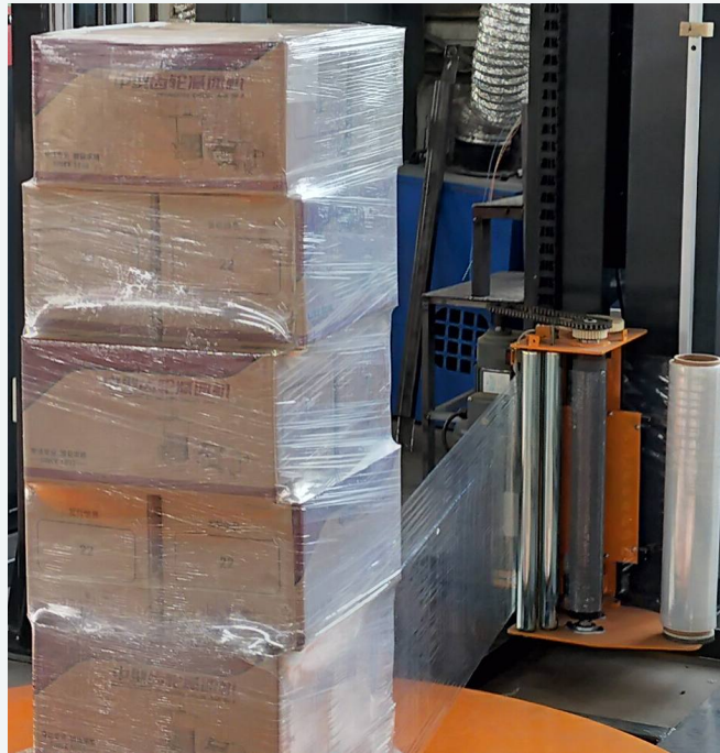
Load reference | Film application around stacked cartons
