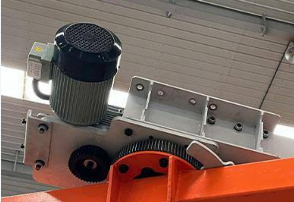
Rotary drive, gear and mounting bracket detail.
